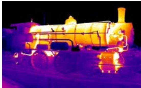
Thermal image of steam locomotive made by IR camera KT-384 from Sonel S.A.
